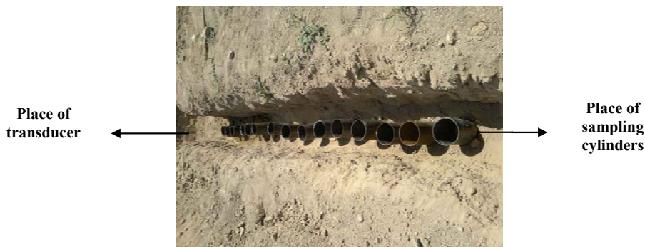
Figure 3. Positions of cylinders inside soil profile before filling with loosened soil
