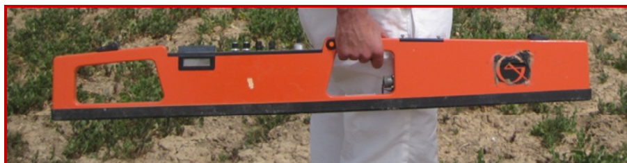
Figure. 1. Electromagnetic Conductimeter EM 38 in vertical position
