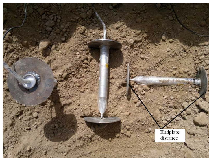
Figure 2. Position of transducer inside soil profile left to right, vertical, lateral and longitudinal
